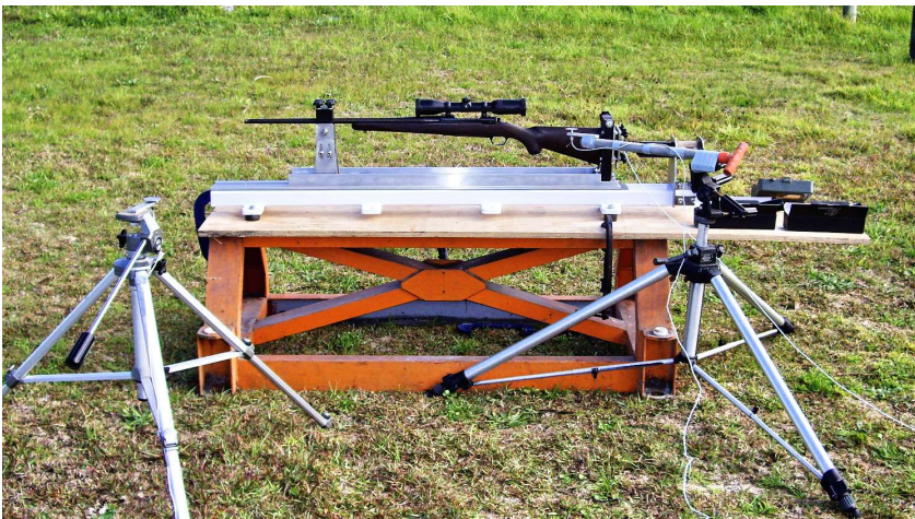
The setup with the weapon clamped in the recoil jig and the two overpressure sensors.
